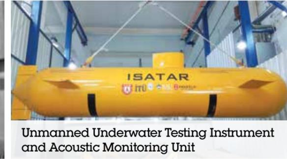
Unmanned Underwater Testing Instrument and Acoustic Monitoring Unit
